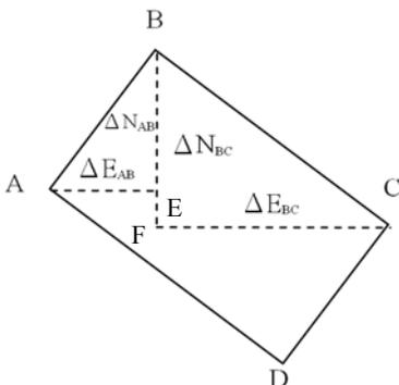
15.  $\phi_{AC} = \phi_{AC} + \angle A = 270^\circ + (250^\circ - 130^\circ) - 360^\circ = 30^\circ$
